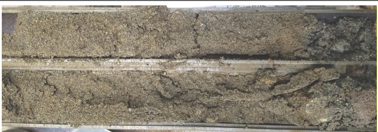
Plate 3. SPT sample of pre-Olympia Coarse Grained Deposit, PG-3, S-4, 7.5'.
